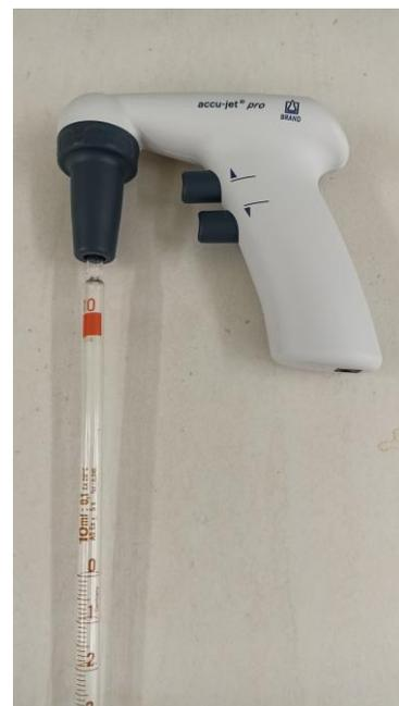
Picture 2 – Pipettor with attached pipette.
