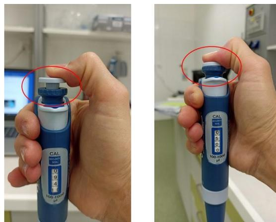
Picture 4a/4b – First/second position of pipetting.
