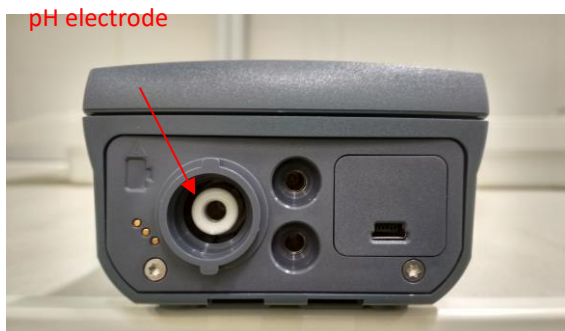
Fig. 2: Connection of pH electrode.
