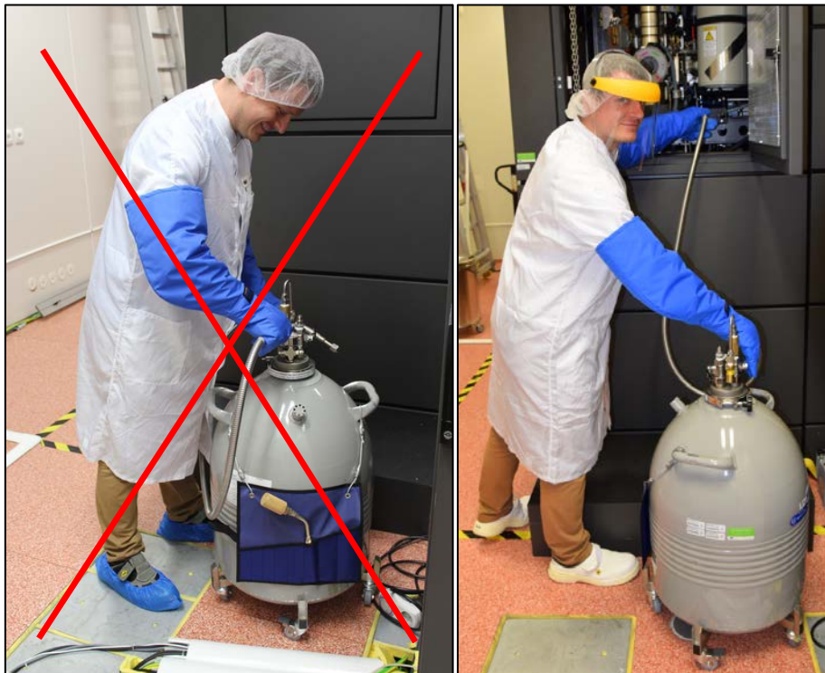
Figure 32: Dealing with liquid nitrogen – TEM laboratory (on the left picture the face shield is missing)
