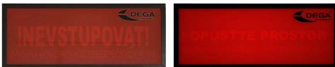
Figure 34: Signal panels are activated when the alarm level is reached.
