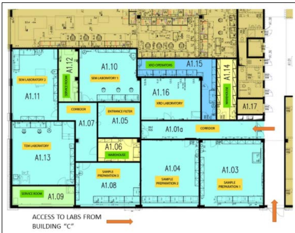
Figure 22: Building A – Entrance path to the cleanroom
