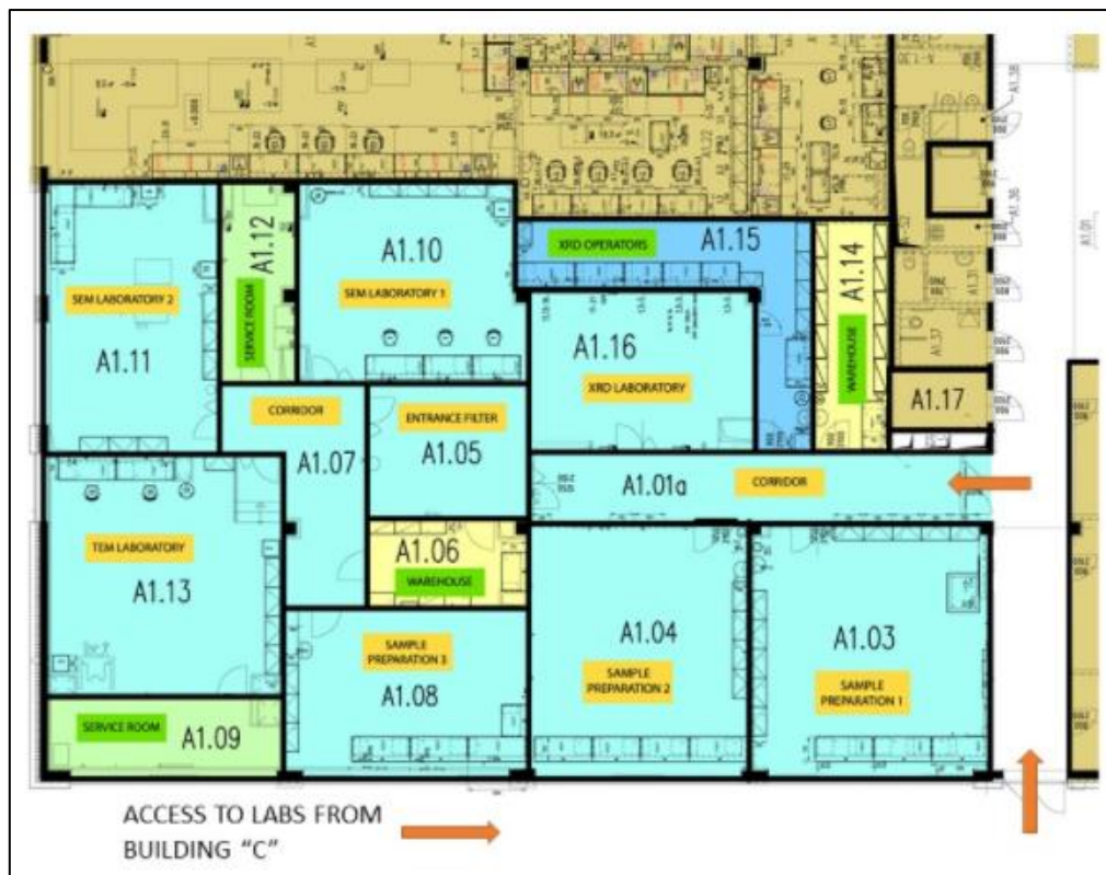
Figure 22: Building A – Entrance path to the cleanroom
