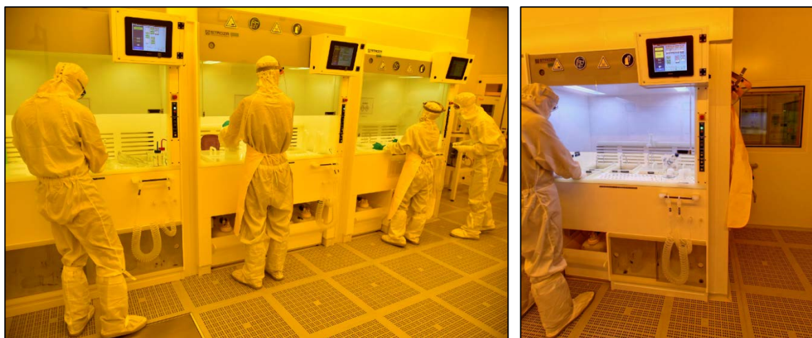
Figure 24: Fume Hoods in the Chemical lab
