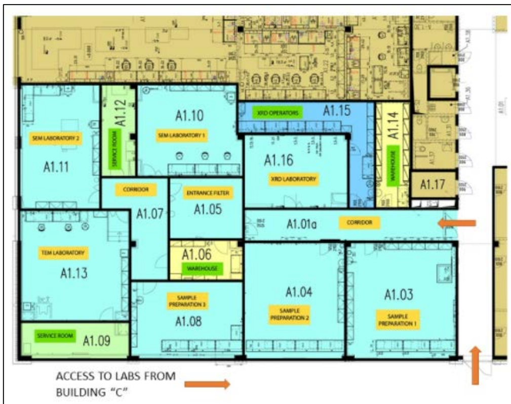
Figure 19: Building A – Entrance path to the cleanroom
