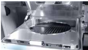
Fully automated 8 inch loadlock
