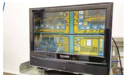
Screen view after cutting – the cut-width is about 50 µm
