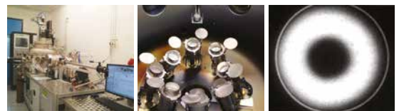
Planar magnetron target using permanent magnets to supply the magnetic field (after Wasa and Hayakawa) [1].
