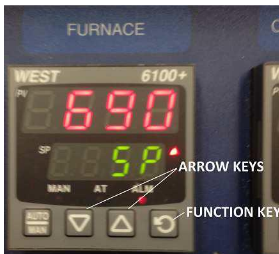
Figure 5: Setpoint controller explanation.
