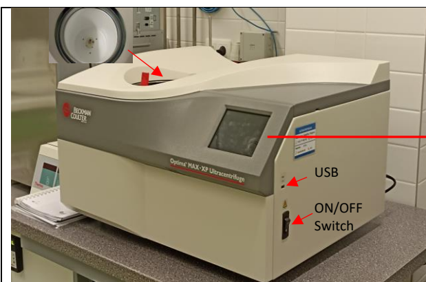
Fig. 7: Ultracentrifuge Optima MAX-XP. Details: the drive hup, USB and Switch ON/OFF.
