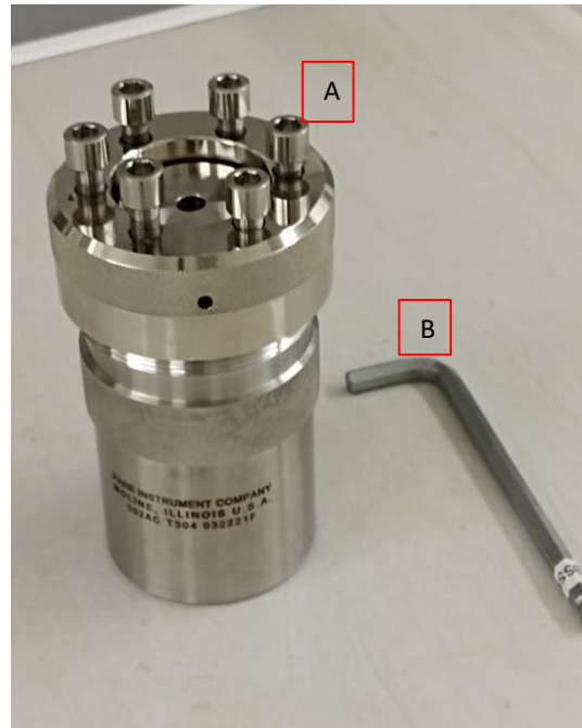
Picture 2: Completed the acid digestion vessel (hydrothermal reactor) (A) and vessel key (B).
