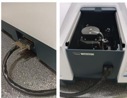
Fig. 1: Connection of the integrating sphere.
